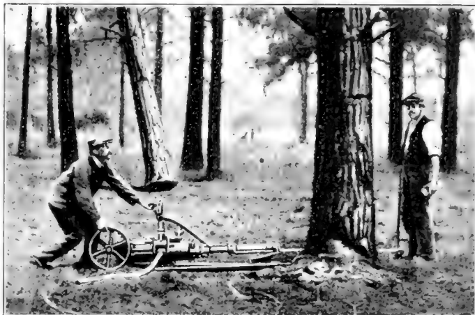
One of these steam-operated sawing machines attended by a gang of four men will perform more work in an eight-hour day than thirty woodmen
